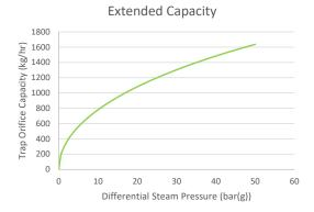
Maximum discharge capacity for Opal Trap at saturation temperature.\*
